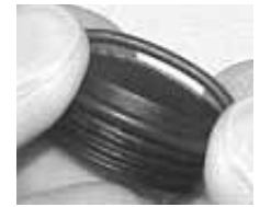
Fig. 102 - INSTALLING COVER O-RING
